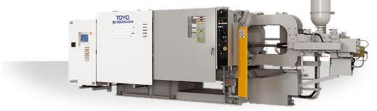
Incorporates the latest microprocessor control system "SYSTEM 500" for greatly enhanced machine operability
