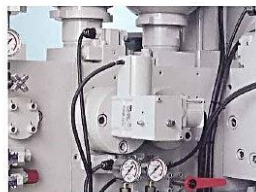
Electric injection flow control valve Effects remote control of the injection speed adjustment. Also automatically corrects speed and pressure rise time.
